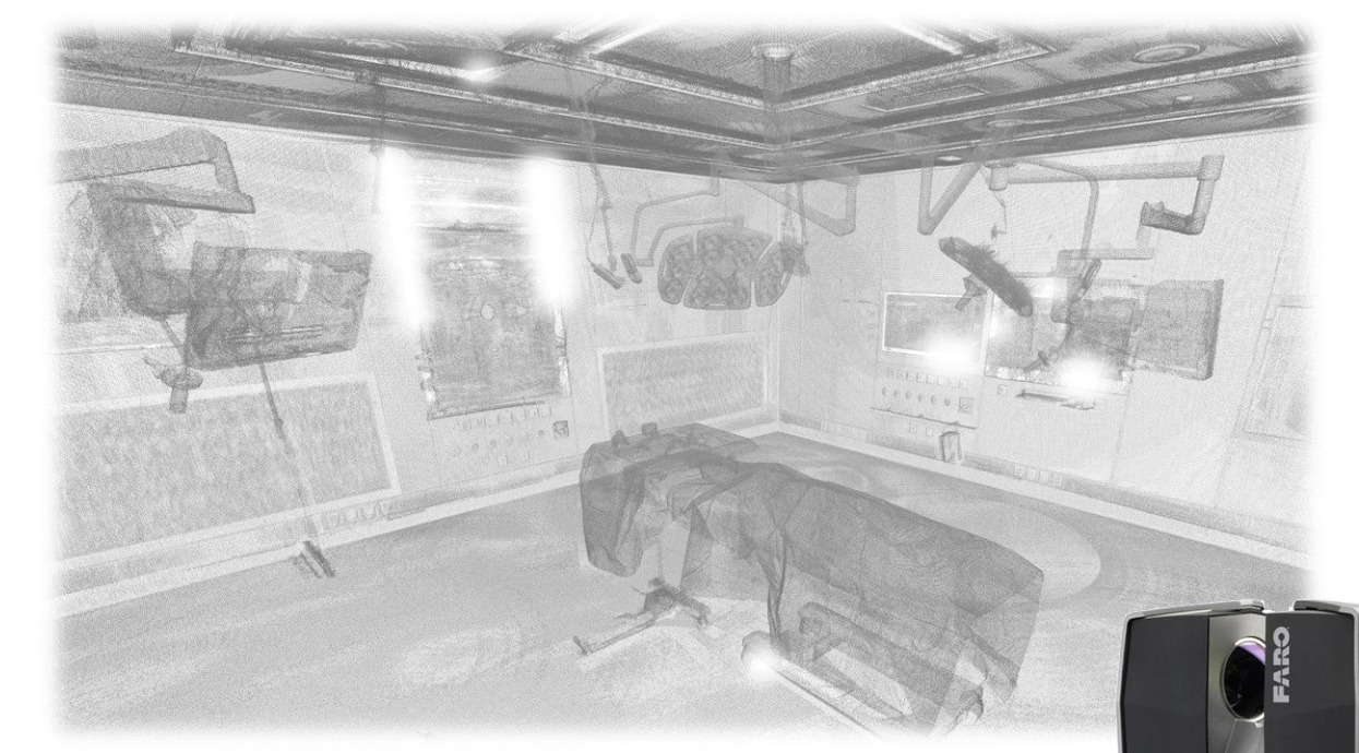
Spatial Reference Frame A fusion of 8 high-resolution point clouds obtained from a laser scanner serves as a spatial reference.
